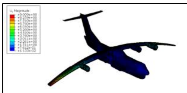
Figure 9 Symmetric First-Order Mode of the Entire Aircraft
