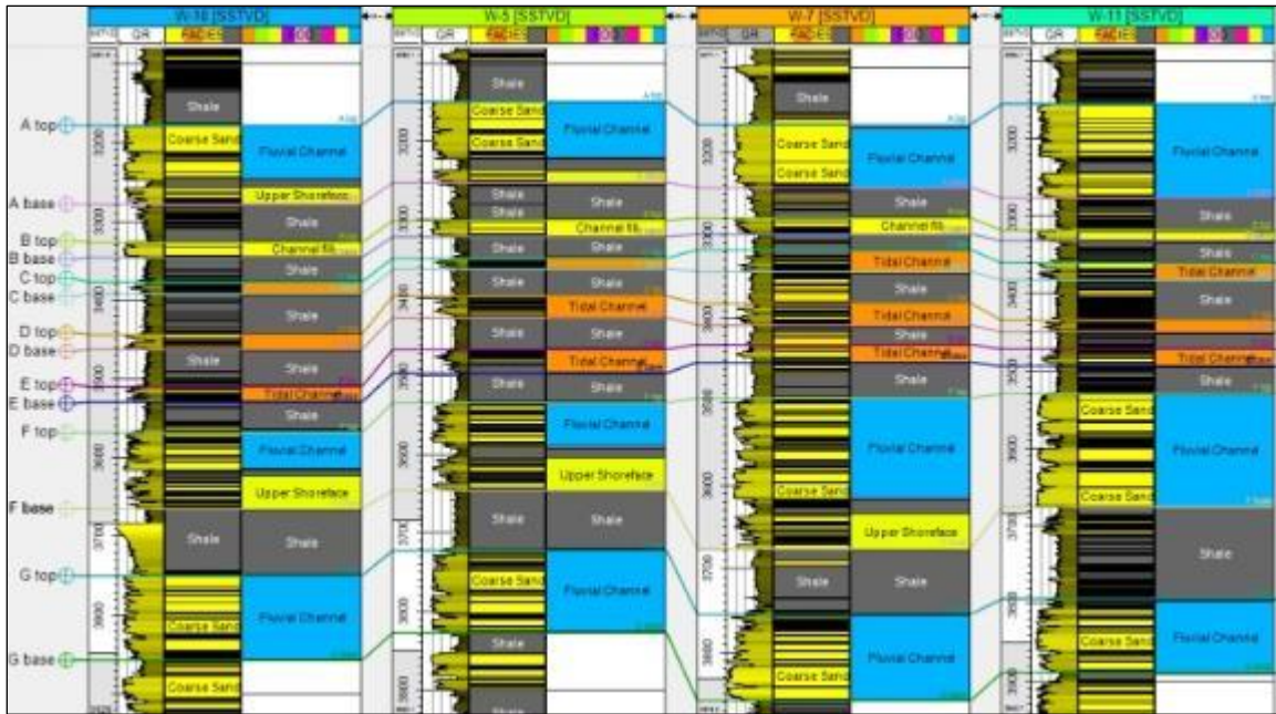
Figure 4 Facies and environment of deposition inferred for reservoir sands within the field
