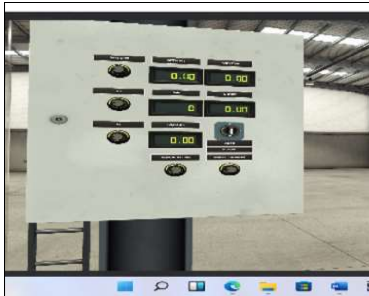
Figure 2 Control Panel Design in Factory I/O
