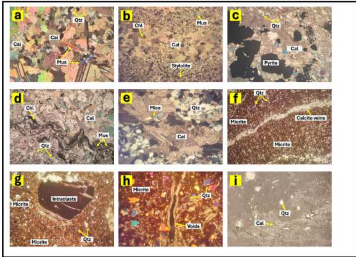
Figure 6 a) Crystalline limestone, b) Banded limestone, c) Massive limestone, d) Calc schist limestone, e) Massive limestone, f) Arillaceous limestone, g) Micritic limestone, h) Micritic limestone, i) Lime kankar
