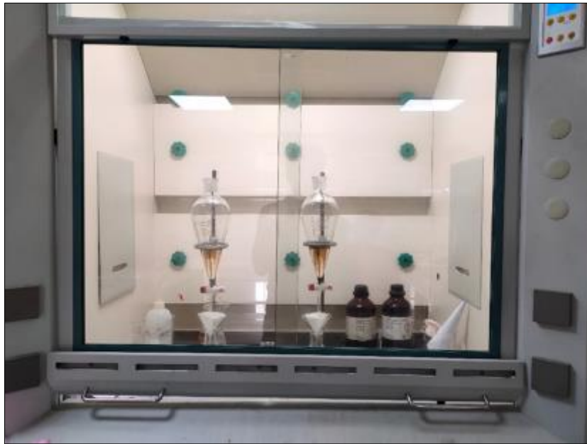
Figure 12 Heavy mineral separation using tetra-bromo ethane
