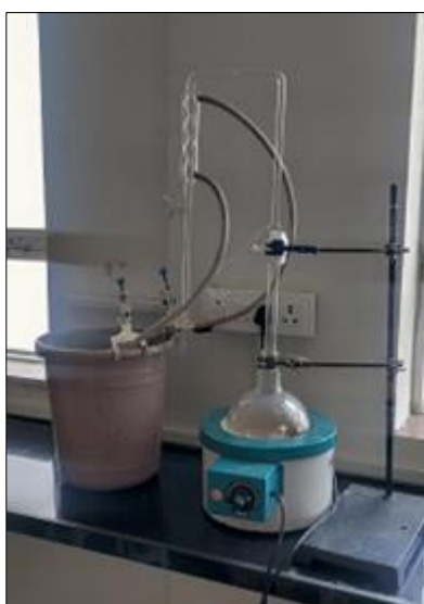
Figure 3 Separate of essential oil from Plumeria Alba flowers by hydro distillation in a Clevenger- glass apparatus
