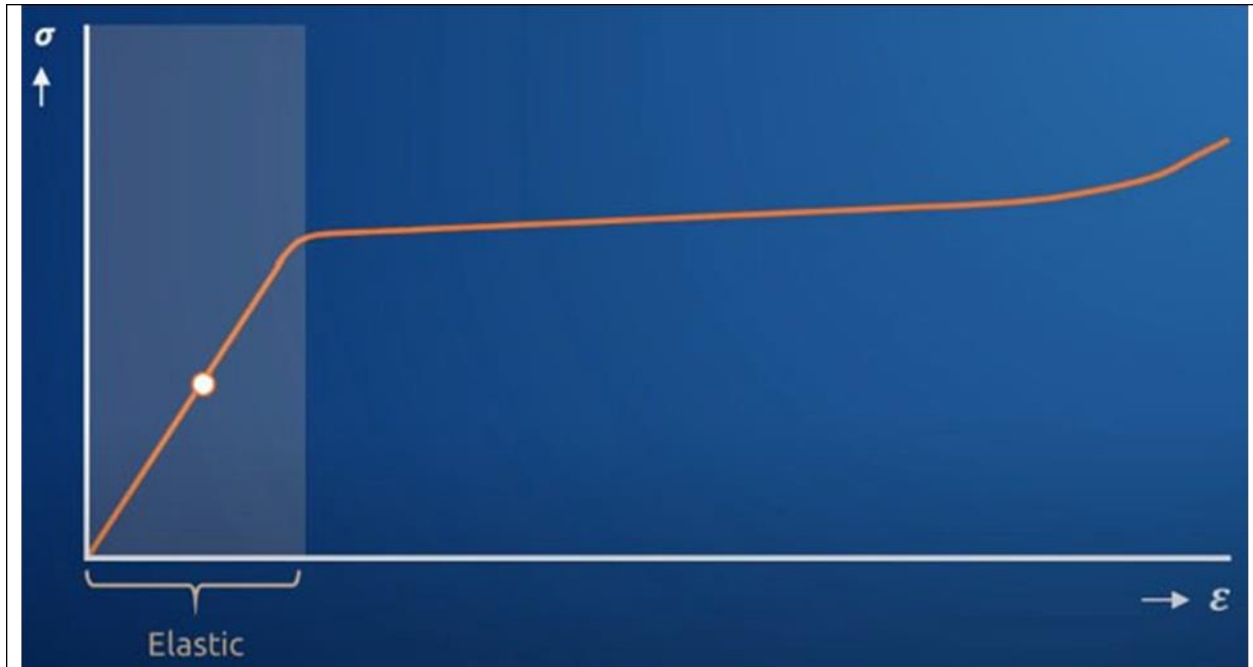
Figure 5 Bolt Stress-strain curve showing typical yield behaviour
