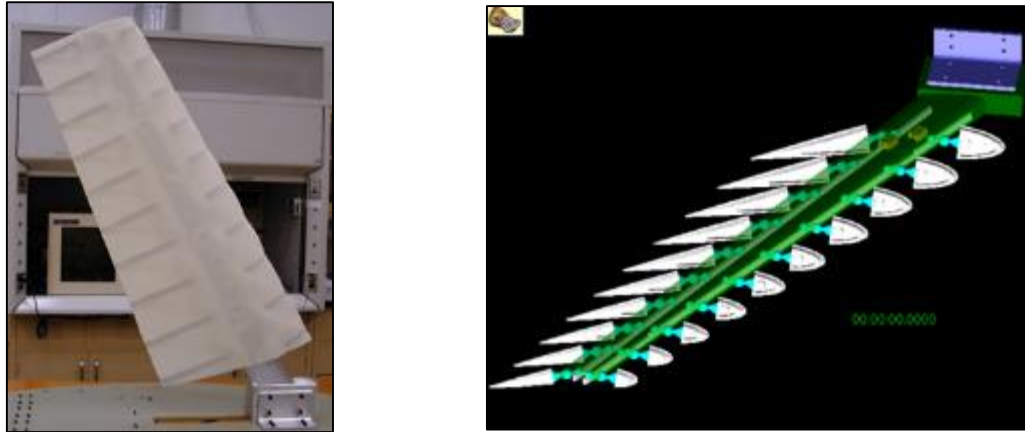
a) LaRC Fish Bone morphing wing prototype [8] b) Dynamic Analysis and Design System model [8]
