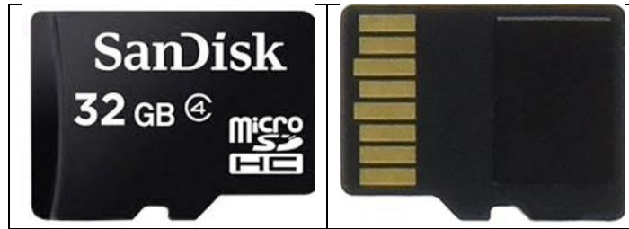
Figure 7 Micro SD card front and back view
