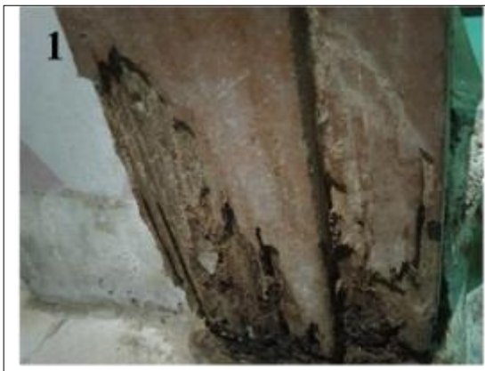
Figure 1 Damage caused by Termites to a part of wood furniture in domestic
