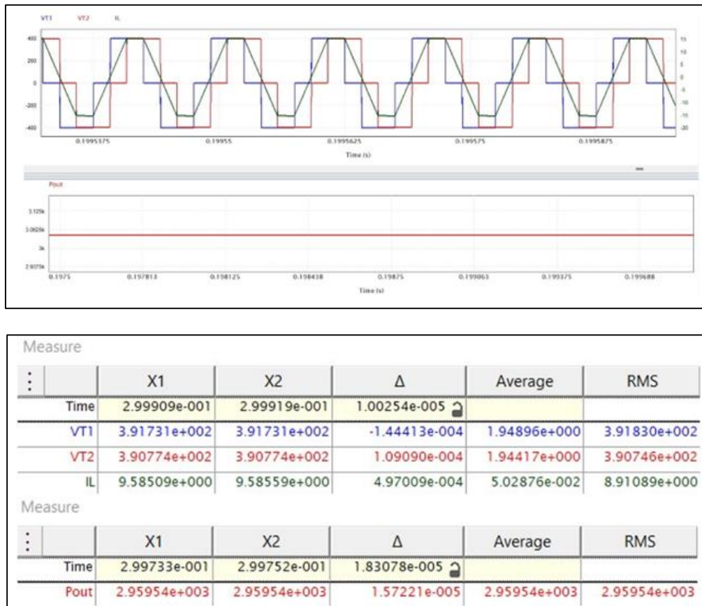
Figure 13 Primary and referred secondary transformer voltage V_{T1} and nV_{T2} and respective inductor current i_L and the output power at V_o = 400 V with SPS Modulation
