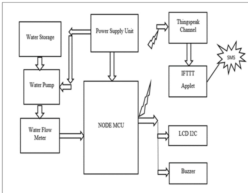
Figure 1 Block Diagram
