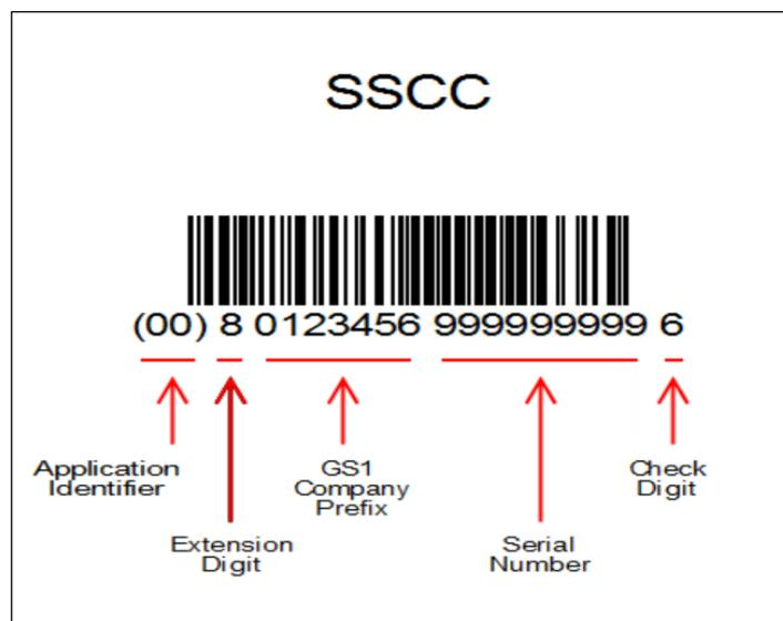
**Figure 4** SSCC Barcode on Tertiary Packaging
