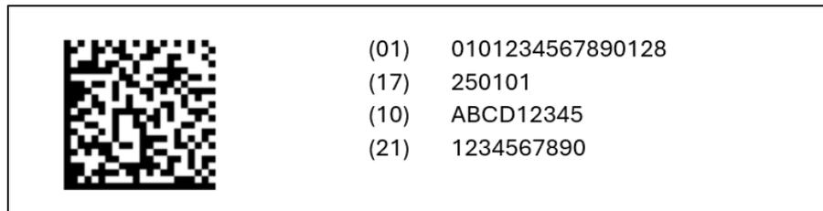
Figure 1 Data Matrix Barcode on the Primary Packaging
