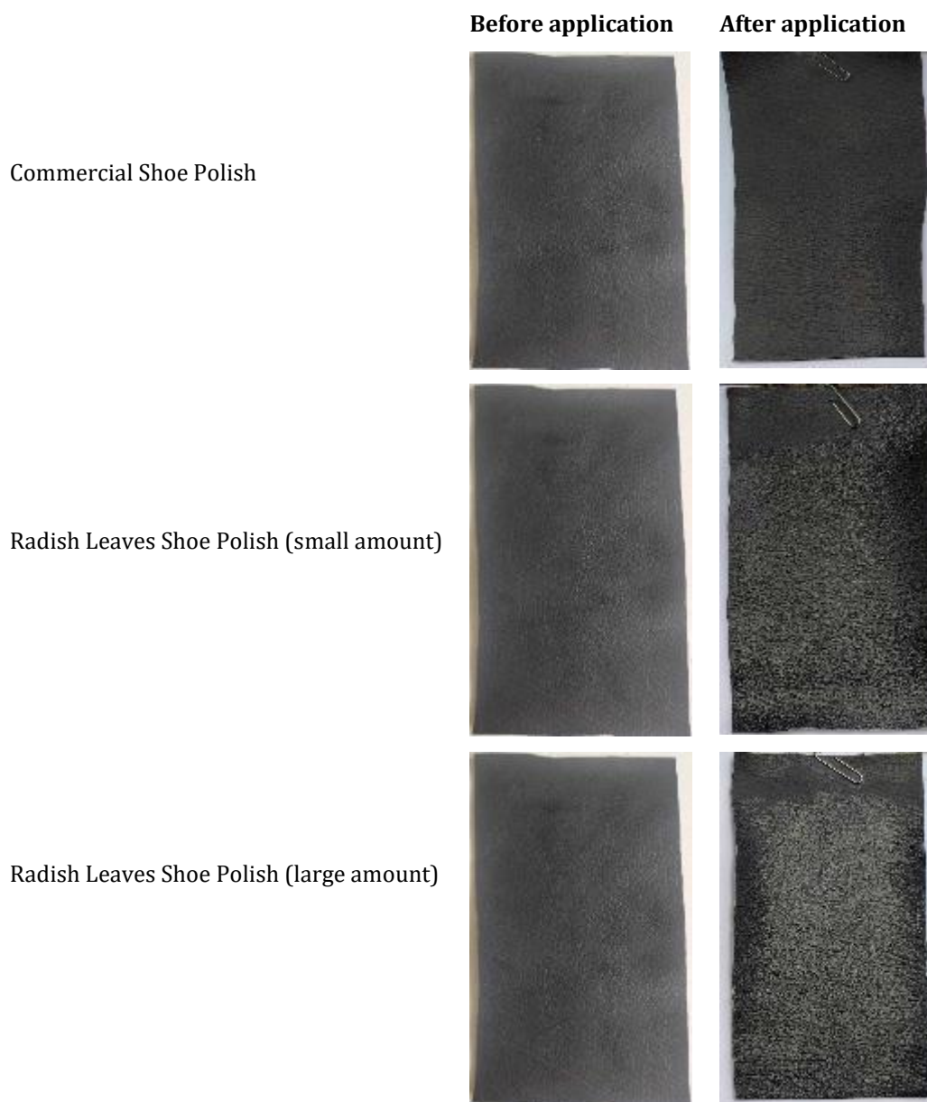
Figure 6 Checking the ability to resist dust over twenty four (24) hours
