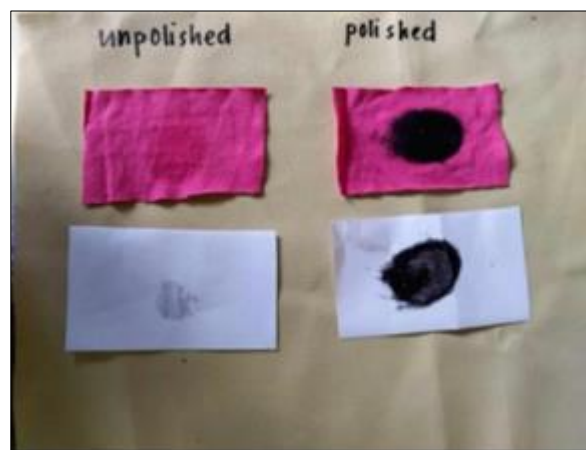
Figure 5 Three minutes after dropping an ample amount of water in polished and unpolished cloth and paper
