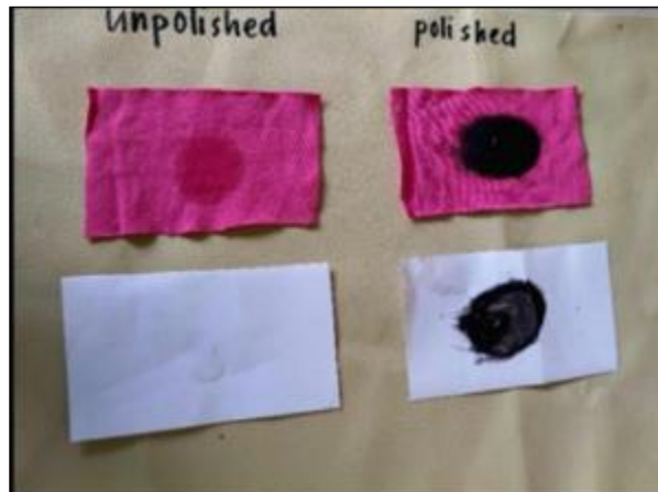
Figure 4 Checking the ability to repel water using paper and cloth
