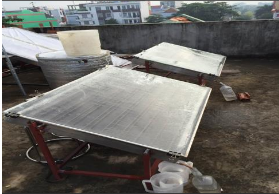
Figure 2 Experimenting in parallel with two distillation equipment using solar energy in a stepped solar still
