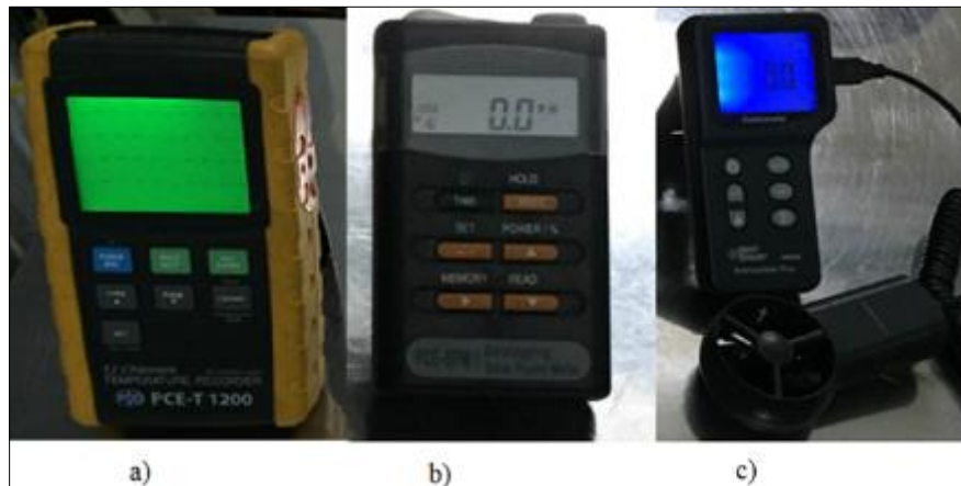
Temperature metter b) Solar power Meter c) Digital anemometer
